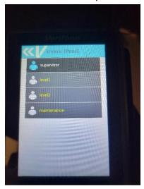
6. Once logged in press the 3 button to select update. Then select "Serial" in this menu. (This is a guide for USB the Verifone units use the serial option to update) From here select "COM 5" then "Auto"
